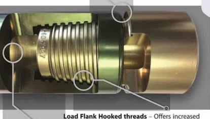
torque capabilities verses typical HDD threads by reducing eccentric loading on the box.
